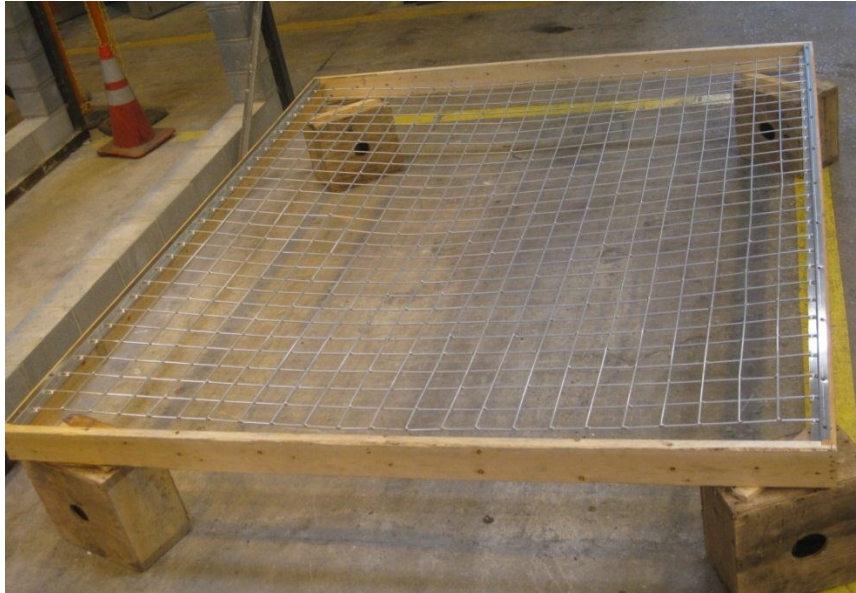
Photo No. 1 Fall Guard/Security Grill
