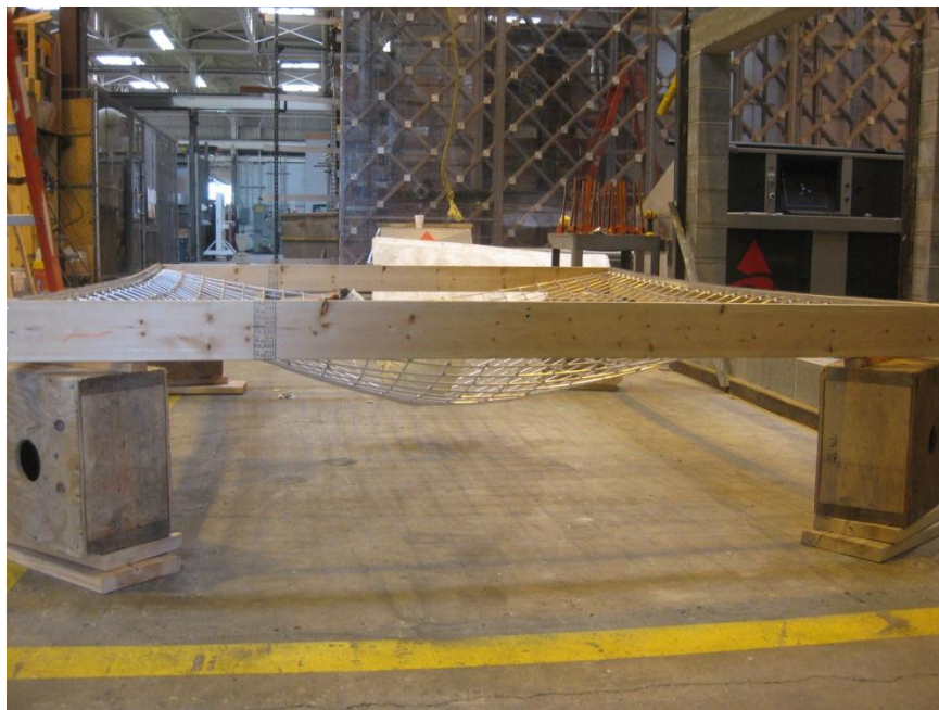
Photo No. 6 After 4 ft. Drop
