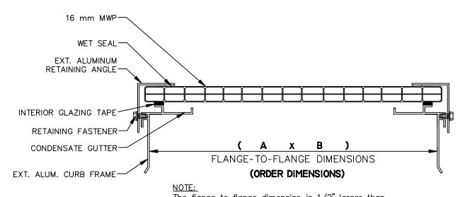
The flange-to-flange dimension is 1/2" larger than the outside dimension of curb, unless directed otherwise
