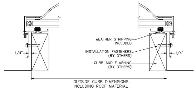
**CURB MOUNT-GLASS; THERMALLY BROKEN FOR FLAT ROOF APPLICATION - SPECIFICATION:** Curb Mount-Glass; Thermally Broken, as manufactured by ORCA Manufacturing, Inc., with insulated glass unit (Clear tempered over tempered standard, Low-E, tinted or laminated as an option) with a single outer acrylic dome in a welded thermally broken, extruded aluminum sash. Each unit will have a built-in evaporative condensation gutter. Finish in bronze, (white gloss enamel as an option).
