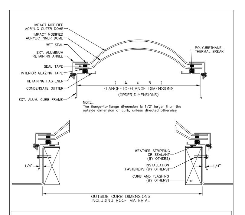
CURB MOUNT-IMPACT MODIFIED ACRYLIC; THERMALLY BROKEN - SPECIFICATION:
